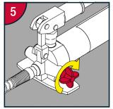
To engage, ensure flow valve is in the closed position.
