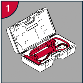
Remove the Hydraulic Assembly from the HDPE storage case.
