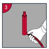
Hydraulic Assembly can be used vertically.
