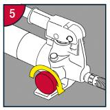
To engage, ensure flow valve is fully closed (turn clockwise to close).
