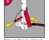
Remove bottom pin and insert ram into ram access chamber.
