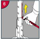
Lift hose to raise ram and inner tube until top plate is close to object surface.
