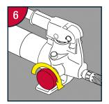
Check flow valve is in the fully closed position (turn clockwise to close).
