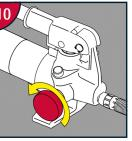
Open flow valve to allow ram stick to retract and inner tube
