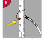
Insert bottom pin through first available hole directly beneath ram.
