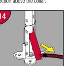
Whilst holding hose, take out bottom pin then lower hose and remove ram.
