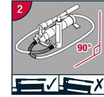
Ensure the Hydraulic Assembly is placed in a horizontal position or it will not function properly.
