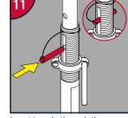
Insert top pin through the available hole in the threaded section above the collar.
