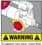
To release ram stick, open flow valve. <u>Never</u> rotate more than one full turn anti-clockwise.
