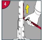
Lift hose to raise ram until ram is as near as possible to inner tube.
