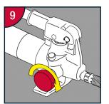
Check pump is horizontal and flow valve is fully closed (turn clockwise to close).
