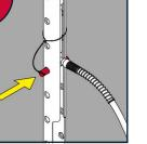
Insert bottom pin through first available hole directly beneath the ram.
