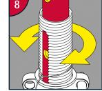
Prior to engaging the pump align holes of inner tube with slot in threaded collar section.
